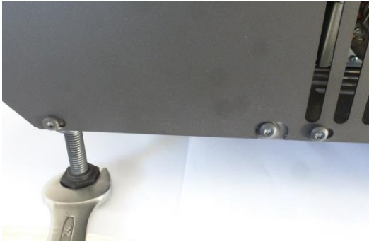
Figure No.4 - Close up of the 24 mm wrench for adjusting the legs
