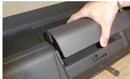
Figure No.2 - Removing the separator
