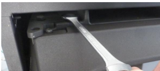
Figure No.9 - Loosening the door support with a 10 mm wrench
